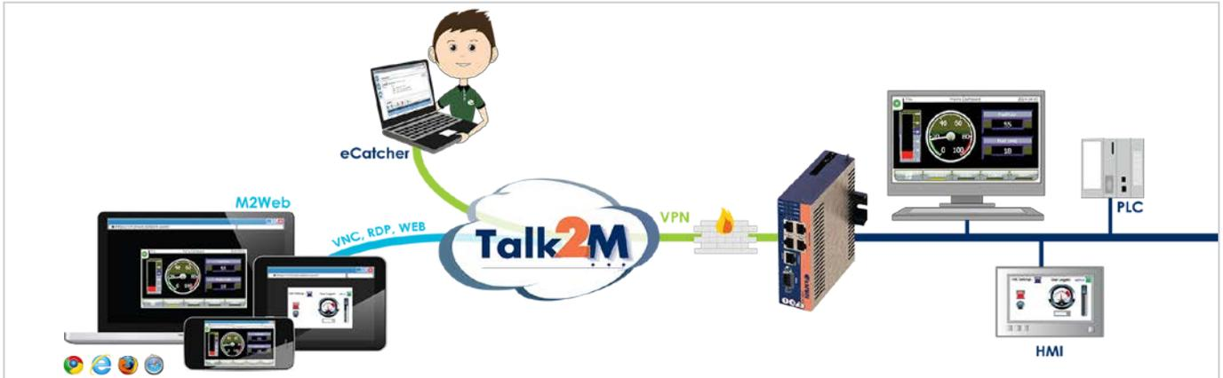
**M2Web** is a standard service of Talk2M, the secure cloud-based remote connectivity solution by eWON. M2Web provides easy and secure access to your remote site using the following technologies:
